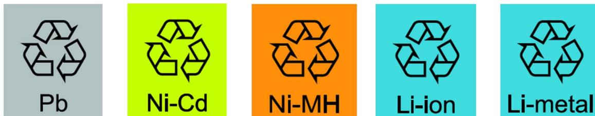
**Figure 6 : Battery markings developed by IEC as published in the draft standard circulated in March 2017**
