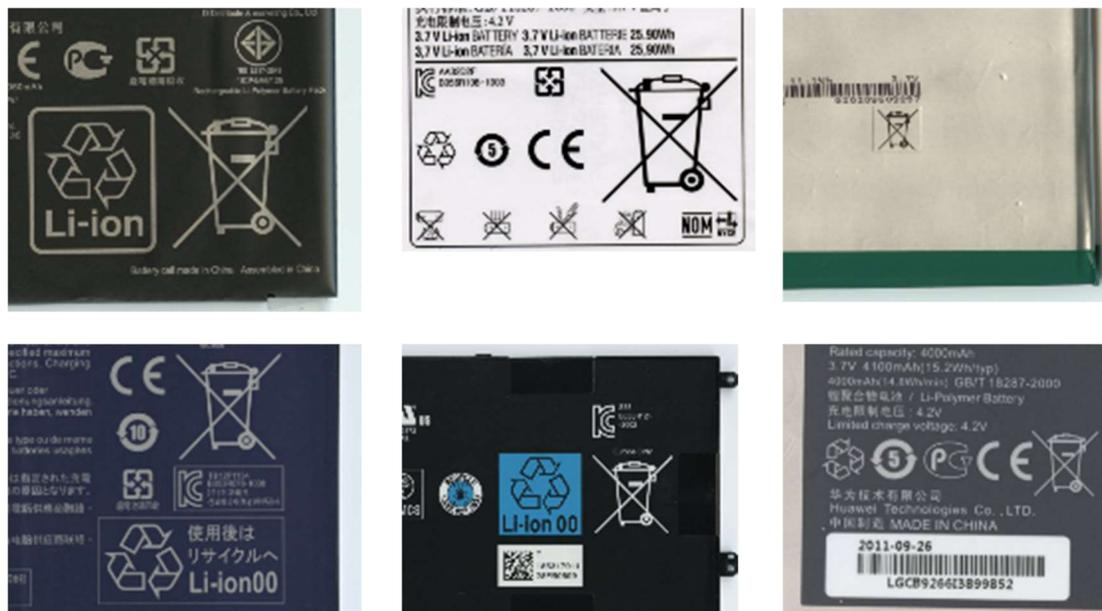
**Figure 3 : Examples of battery marks in current practice**
