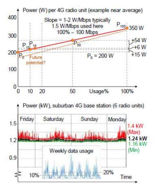
Figure 30: Power and data model for suburban 4G radio unit / base station (based on real data) (Malmodin 2020)
